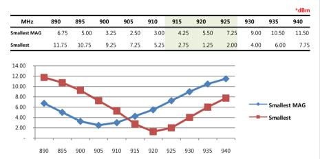
•SMALLEST MAG reads up to 2.0 meters on metal, 20% shorter than SMALLEST. Its read performance varies upon tag location, orientation, direction, RF environments, etc.
